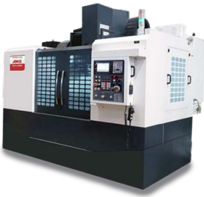
MCV650 vertical machining center
